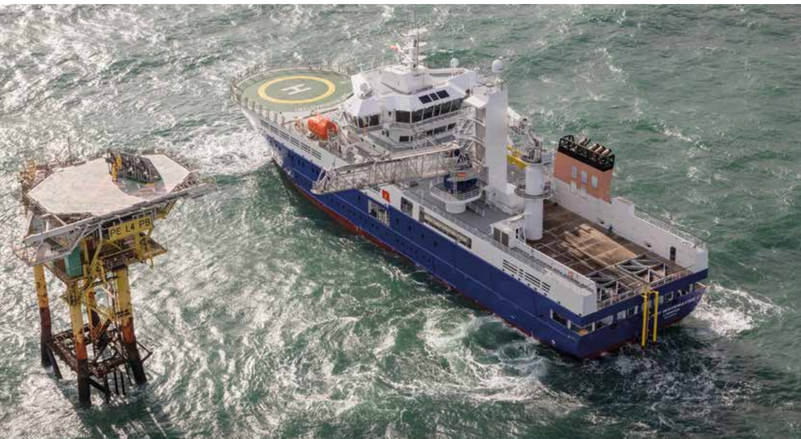
Service Operations Vessels with walk-to-work capability Bibby WaveMaster 1 operating in southern North Sea
